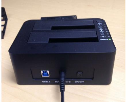
5. Insert original hard drive (to be copied) into slot A and blank hard drive (target to be copied onto) into slot B –docking station lights should turn on to indicate hard drives have been inserted properly
