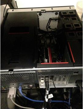
3. Lift up side handles, disconnect hard drive from mounting bracket, and label it (ie. original hard drive)
