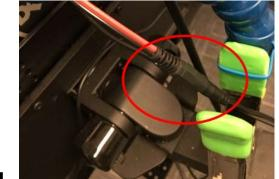
• Unscrew and remove video input/output cable from back of camera; remove microphone from top of camera.
