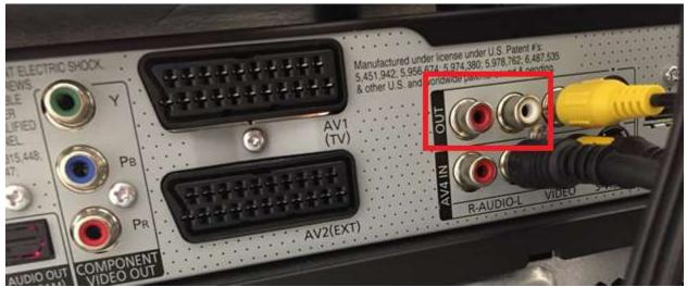
Figure 1. Photo of the back of the DVD player with the RCA output ports boxed in red
