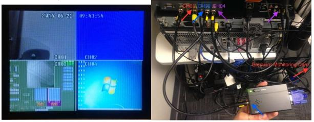
• 2016-11-17: Startech VGA Scan Converter: make sure that the switch on the side of the converter connected to the back of the multiplexor is switched to the left to be set to under scan
