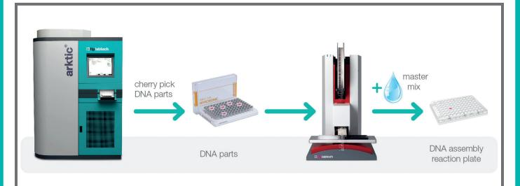
Fig 2. DNA part selection and set up of construct assembly reactions. Example shows how mosquito X1 combines several DNA parts and master mix into a single well (repeated across whole plate in practice).
