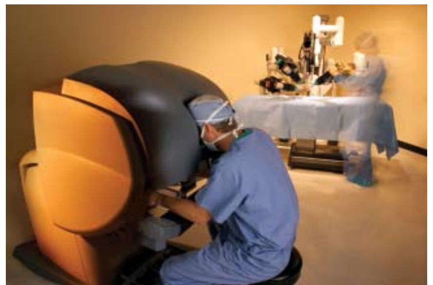
The da Vinci Surgical System, seen here in a photo from Intuitive Surgical, gives surgeons precise control over robotic arms (background) for minimally invasive procedures and a clear view of the operating field.
