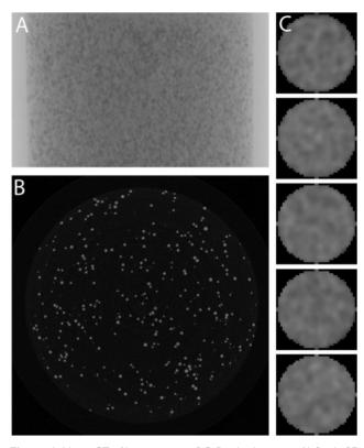
Figure 4: Micro-CT of homogeneous RO Beads phantoms. A) Single 2D projection, B) Slice through reconstructed data, and C) Column of individual beads (~160  $\mu$ m diameter).
