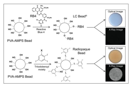
Figure 1: Comparison of LC Bead and Radiopaque LC Bead (RO Bead) dye attachment. Acrylamido polyvinyl alcohol-co-acrylamido-2-methylpropane sulfonate hydrogel (PVA-AMPS) beads are reacted with Reactive Blue 4 (RB4) to make LC Bead visible (blue) to the user. RB4 is substituted with a triiodobenzyl moiety via a linker (L) for RO Beads which imparts a slight yellow color and importantly renders them visible on X-ray.
