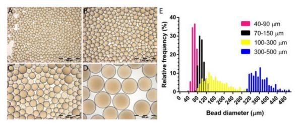
Figure 2: Optical micrographs of RO Beads. A) 40-90 µm, B) 70-150 µm, C) 100-300 µm and D) 300-500 µm. E) Relative frequency distribution of RO Beads size measured with an optical microscope (N = 200-214).
