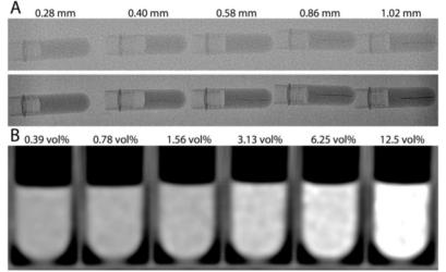
Figure 5: A) 2D X-ray images of RO Beads line phantoms. Standard fluoroscopy (top row) and X-ray single shot (bottom row) show a series of microfuge tubes with horizontal line phantoms mimicking blood vessels of various inner diameters. B) Multidetector computed tomography of RO Beads phantoms with a six factor serial dilution of RO Beads ranging from 12.5 to 0.39% sedimented bead volume (vol%).
