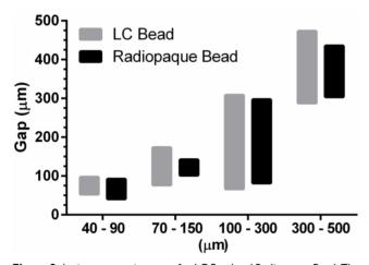
**Figure 3:** *In vitro* penetration assay for LC Bead and Radiopaque Bead. The bar graphs depict penetration potential according to bead size. The bottom of the bar is the maximum penetration of the bead and the top of the bar is the trailing edge of a bead population (0.5 mL aliquot of sedimented beads). The maximum penetration and the the trailing edge for each size range was measured and displayed as an average (N=3).
