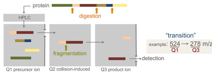
MRM is highly specific assay method for detecting analytes of interest utilizing, most predominantly, a triple quadrupole-based mass spectrometer. Q1 is set to transmit only the parent m/z of the peptide, the fragmentation via collisional induced dissociation occurs in Q2, and Q3 is set to transmit this diagnostic fragment only. The specific combination of m/z associated with the parent and fragment ion selected are referred to as a "transition".
