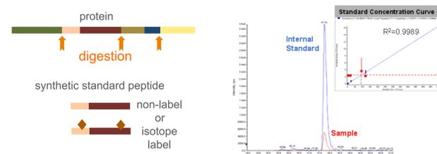
In absolute quantitation experiments, the analyte of interest is used to generate a calibration curve to characterize the MS response of each analyte. This can be done with the analyte alone or with an additional isotope labeled analyte that has identical MS response. A calibration curve is generated and the amount of analyte present in each sample is determined by comparing to the curve.
