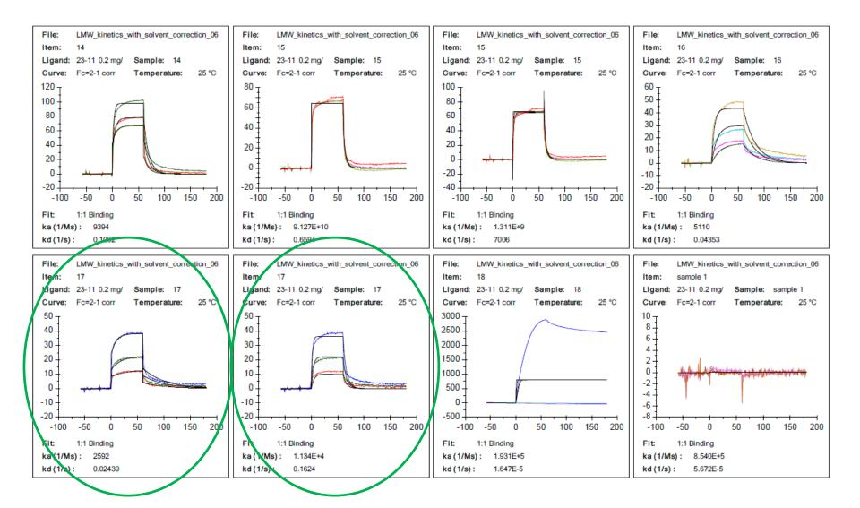
PrP protein was immobilized directly to CM5 chip via amine-coupling; binding of small molecules was monitored in PBS supplemented with 0.05% of Tween 20 detergent and 5% of DMSO.
