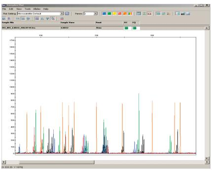
Figure 3. Five-dye chemistry increases the number of markers that can be run in a single capillary, for improved throughput. Above is an example of 18 microsatellite loci co-electrophoresed in a single capillary.
