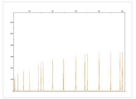
Figure 4. Overlay of 16 GeneScan<sup>™</sup>-500 LIZ<sup>®</sup> size-standard electropherograms shows sizing precision on the 3130 Series Systems.
